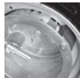
21. If the **spacing** between the wheels is **very large**, **mount both spacer segments** on the **inside** at the **edge** of the coupling case.
