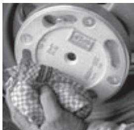
11. To make your Clic dual wheels couple easily, clean the coupling surfaces with a cleaning cloth every time before you mount the dual wheels. The vehicle wheel has now been prepared to accept the Clic dual wheel.
