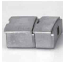
17. You can use the 20 mm and 30 mm spacer segments to set the distance between the wheels. When you have determined the position in which the dual wheels must be mounted with the spacer segments, click the coupling case off the vehicle again. This makes it easier to mount them.
