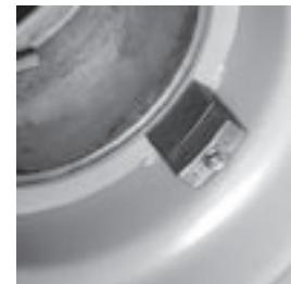
19. If there is **no distance A** between the wheel disk in **Figure 19** and the edge of the coupling case, **mount the two spacer segments** on the **inside** of the edge of the coupling case or on the **outside** of the dual wheel.
