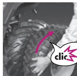
28. As soon as the dual wheel slides in against the vehicle, turn the dual wheel forcefully with momentum against the direction of travel until you hear it clic into place.
