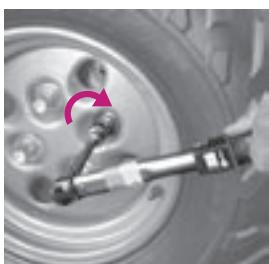
6. Please observe the **tightening instructions** in the operating instructions for your vehicle. The adapter nuts must be **tightened** just as tightly as normal wheel nuts.
