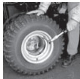
25. First tighten all nuts with approx. half torque, then fully in accordance with Figure 5. To couple and uncouple, it is best to drive your vehicle onto an approx. 30 mm thick plank (included in the Clic Pick-up scope of supply). The tightening moment is 32 Nm (3,2 kg/M) max.
