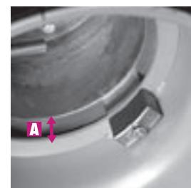
20. When the distance **A** is approx. **20 mm**, **mount the wide spacer segment** on the **outside** and the **narrow one** on the **inside**. Always place the **washer** directly **under** the nut!
