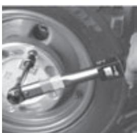
10. Use the Torx wrench T50 provided to tighten the bolts. Tighten them first to half torque and then to full torque as described under **Number 5**. The **maximum tightening moment** is 40 Nm (4.0 kg/M) max. as shown in **Figure 10**.
