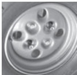
3. Screw 2 adapter nuts onto the exposed bolts in a way that a possible sinking against the vehicle is evident. (Some types of vehicles have flat wheel nuts, in which case the adapter nuts are also flat.) Tighten these 2 nuts to half of the final.
