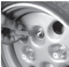
4. Now remove the remaining wheel nuts and **mount** the remaining adapter nuts.
