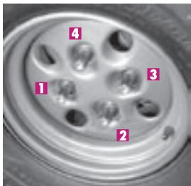
5. Now tighten the adapter nuts to full torque in accordance with this sequence **1, 3, 4, 2**.
