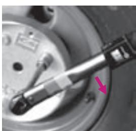
8. **Tighten** the **bolts**, first to half torque and then to full torque as described under **Number 5**. The **maximum tightening moment** is 72 Nm (7,2 kg/M) max.
