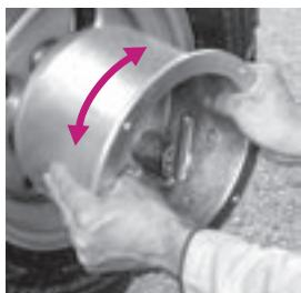
14. Now push the centre pin into the centre hole and press the coupling case against the vehicle. Then turn it in either direction until it slides in against the vehicle.
