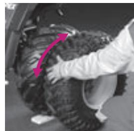
27. After you have moved the centre pin into the centre hole, press the dual wheel against the vehicle with both hands and turn it in either direction at the same time.
