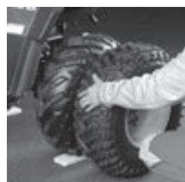
29. Attention! Please make sure that the dual wheel is seated tightly by checking to turn it forcefully to the front. The dual wheel is correctly coupled only when it fits absolutely tight and cannot be turned.
