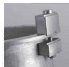
22. The **edge** on the **spacer segments** will hold them in the **correct position**. Always mount them in such a way that the surfaces lie completely on **each other**. The **guide edge** fits onto the **edge** of the coupling case on the **outside**.
